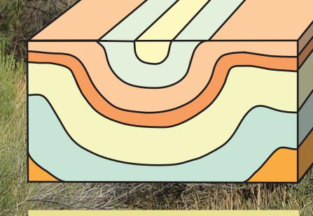
Syncline: The center of the fold is bent downward. On the top surface, the youngest beds are in the middle.
